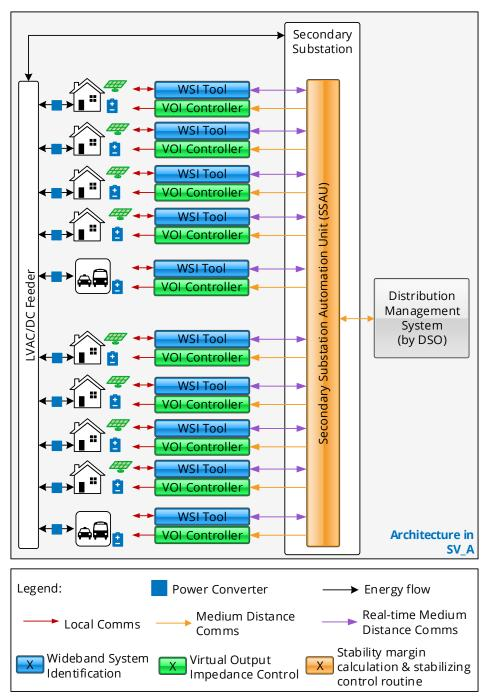
Figure 6. Voltage control architecture in SV\_A
