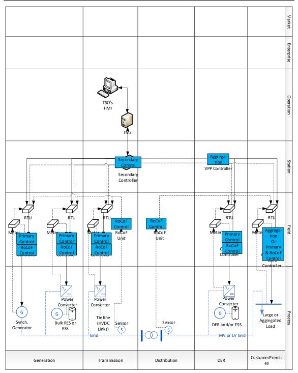
Figure 11. SGAM Function Layer for SF\_B on top of the Component Layer
