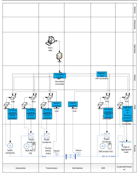
Figure 9. SGAM Function Layer for SF\_A on top of the Component Layer
