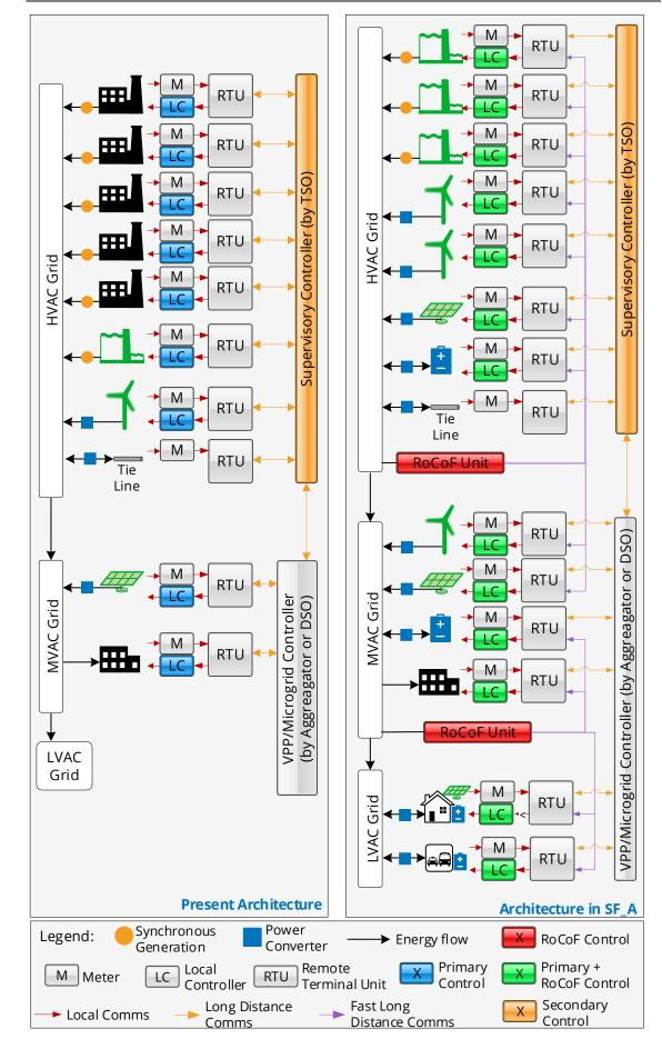
Figure 4. Frequency control architectures today and in SF\_A
