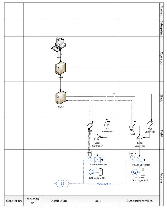
Figure 12. SGAM Component Layer for SV\_A
