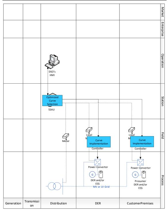
Figure 15. SGAM Function Layer for SV\_B on top of the Component Layer
