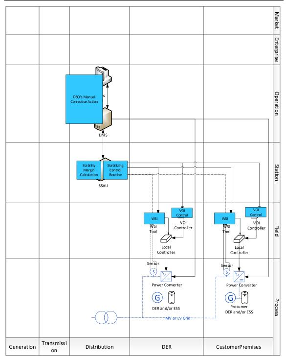
Figure 13. SGAM Function Layer for SV\_A on top of the Component Layer
